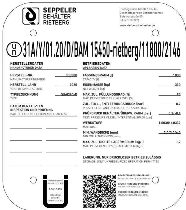
Fig. 1 -1: Example of a name plate for an IBC container
